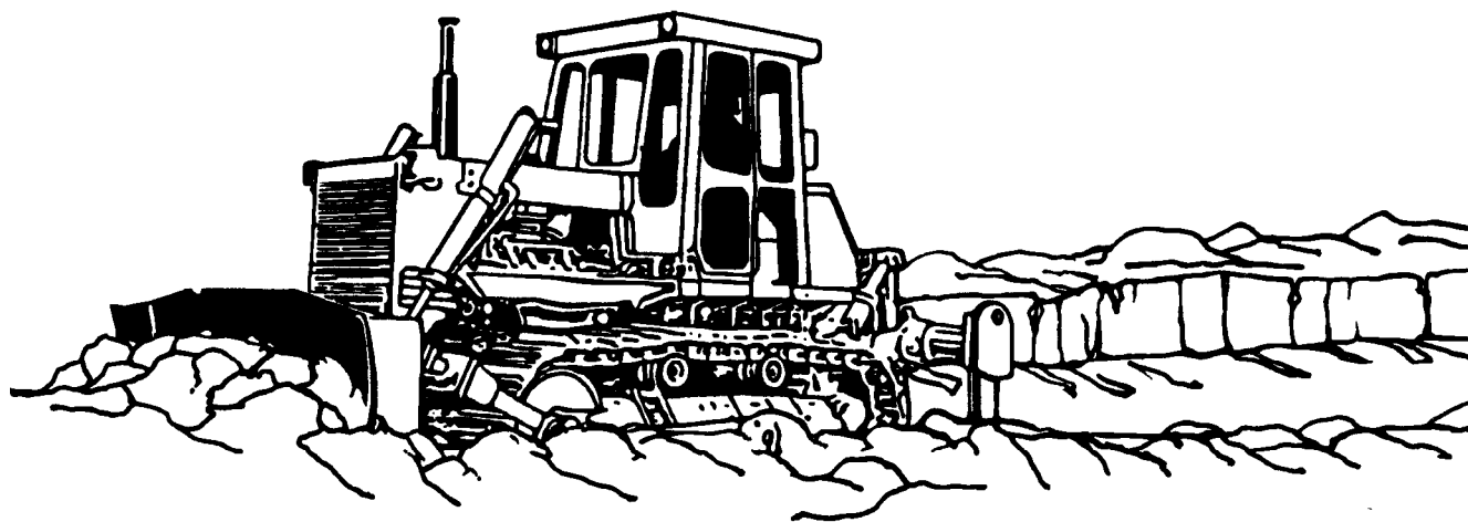
Figure B-2. Dozer trench.
